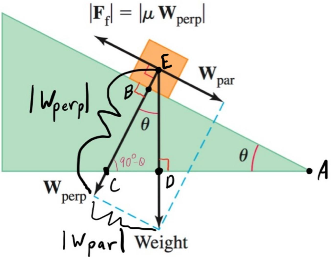
$$(14) \quad \angle ACB = 90^\circ - \angle BAC = 90^\circ - \theta \text{ and}$$
